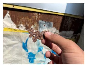
IMAGE 1.17: DELAMINATING STEEL @ PROBE #4
